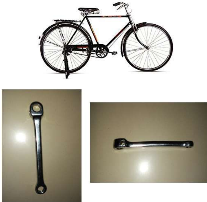
Fig. 1.2 Existing Bicycle crank Component (Hercules Atlas Roadster Bicycle and crank component)
