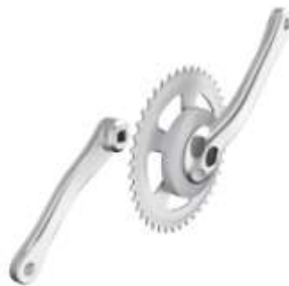
Fig. 1.1 Bicycle crank with chain sprocket
